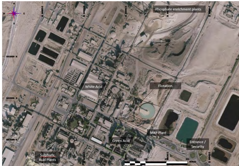
Figure 15.4: Rotem Process Plant Layout
