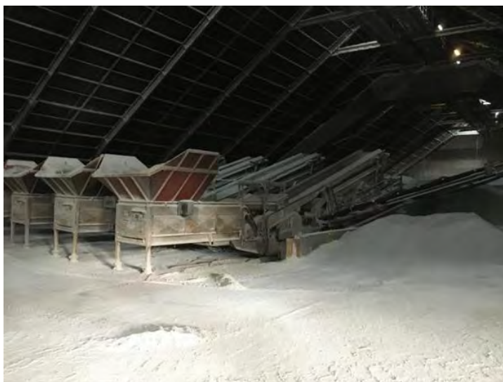
Photo 14.2: Kearton's Building with Mobile Screens and Conveyors at Boulby
