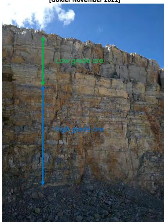
Figure 6.32: Upper Layer Profile in Block #3 [Golder November 2021]
