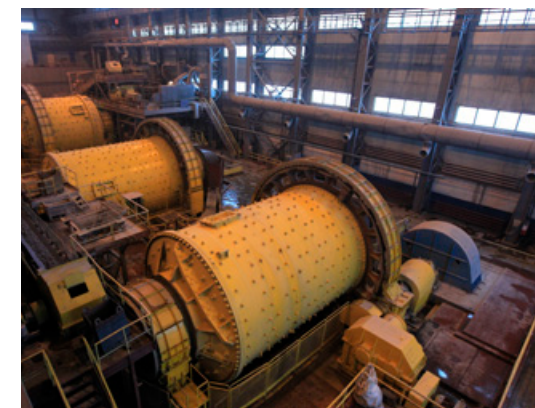
Olimpiada mine. Sulphide ore processing Grinding equipment of ore pretreatment workshop at Mill No. 3. Crushed ore is supplied by a conveyor belt to the SAG mills.
