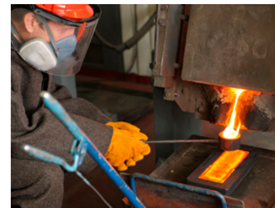
Olimpiada mine. Gold smelting The gold is smelted in the induction furnace. The smelting process lasts for 3 – 3.5 hours at a temperature of 1,200C, following which gold bullions are drained.
