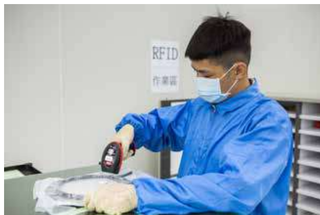
RFID scanning process for real-time parts monitoring
