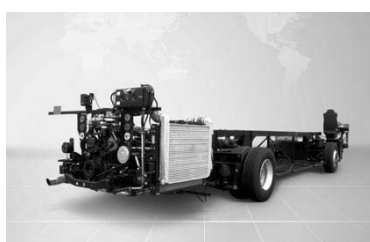
Yutong 11.7M Diesel Coach Chassis (AT)
