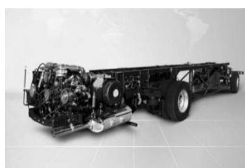
Yutong 11.7M Diesel Coach Chassis (MT)
