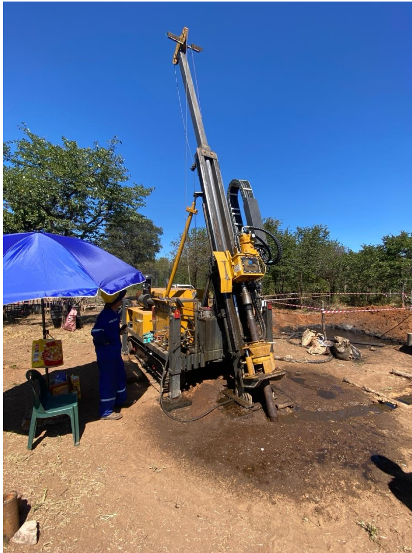
Figure 1: Diamond drilling underway for metallurgical test work at Dokwe North, utilising a drilling rig contracted by Xinhai under the terms of the MST Agreement
