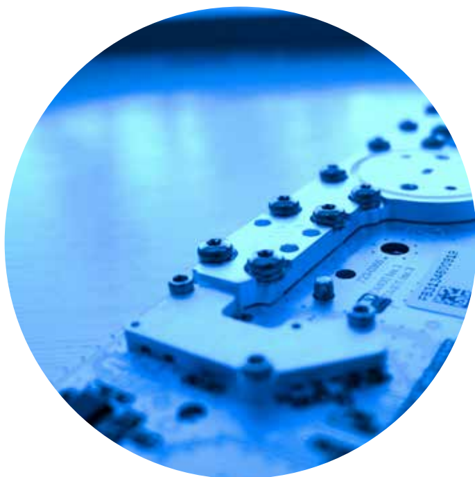
Pictured: E-band transceiver with surface mount diplexer
