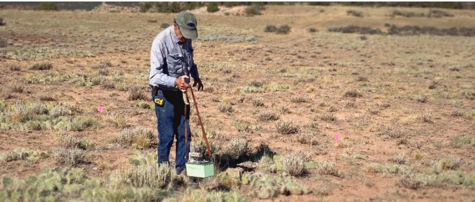
▼ Photo 4: Collecting background Scinotometer readings over proposed drill pads at the Wedding Bell Project (2024)
