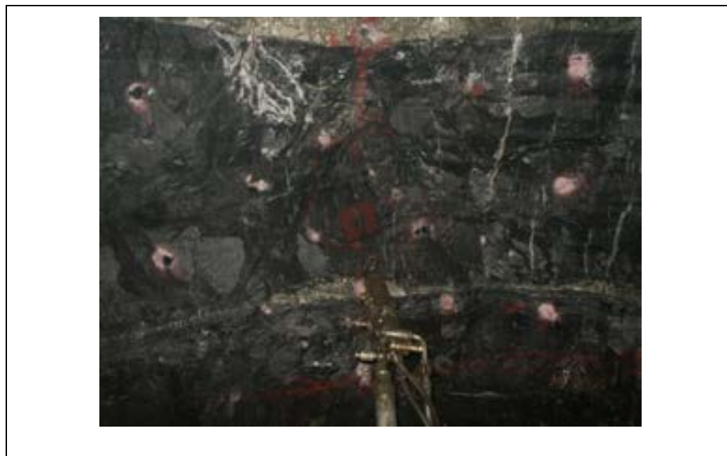
Figure 56: Example of A Pneumatic Rockdrill Drilling the Development Face
