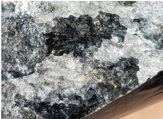
Gold mineralisation in metallurgical samples. Field of View Left: 30mm, Right: 10mm.
