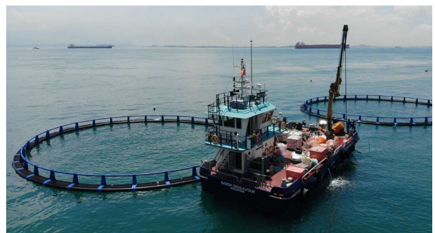
Barra Endeavour was used to deploy the new farm anchors and mooring system, cages and nets. Harvesting and fish transfers are also part of its designed capabilities.
