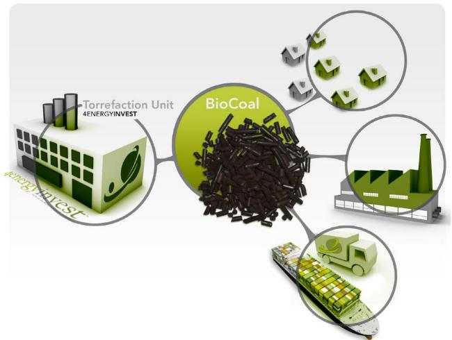
BioCoal is wood processed through a torrefaction unit and then pelletized. BioCoal is a solid enhanced biomass fuel in terms of energy density (almost twice the energy density of wood sawdust pellets (traditional wood pellets) and equivalent to the energy density of fossil coal used in coal fired power stations by utilities). BioCoal aims to displace some fossil coal.
